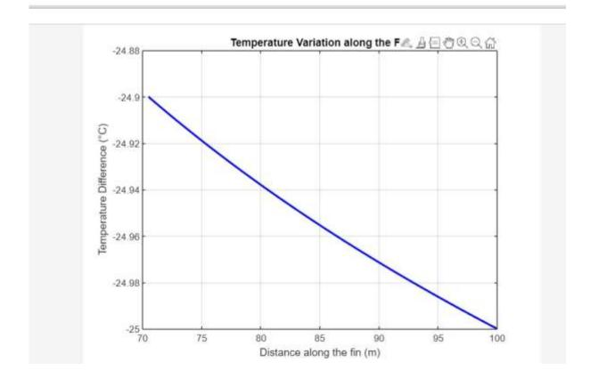
This script defines the differential equation for heat conduction along the fin and uses the ode45 solver to find the temperature distribution along the fin. The script then calculates the temperature difference with respect to the ambient temperature and plots the temperature variation along the fin.
